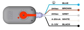
To control the opening and closing of the zone valve through the actuator, simply connect the blue cable to neutral, the brown cable to phase and the black cable to the 0-10V control unit (or the white cable if the regulation is 4-20mA). The grey cable is used to invert the starting point of the actuator and, as far as our applications are concerned, we suggest to leave it always under power.
