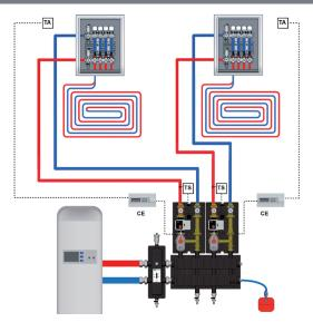
The circulation pattern shows how to install the booster units in the central heating room.
